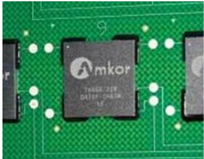
**Figure 3.** Edgebond adhesives typically deposited around corners.
