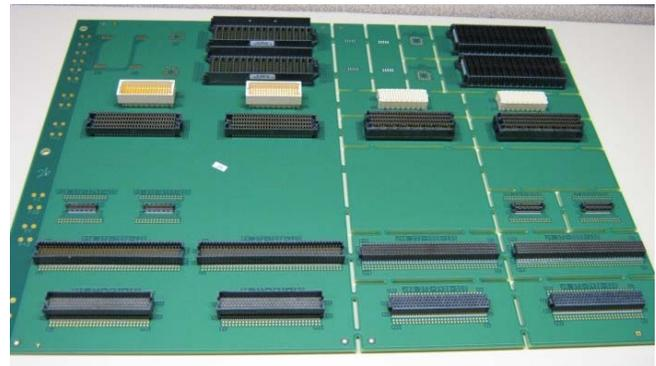
**Figure 7:** As-Assembled Test Vehicle
