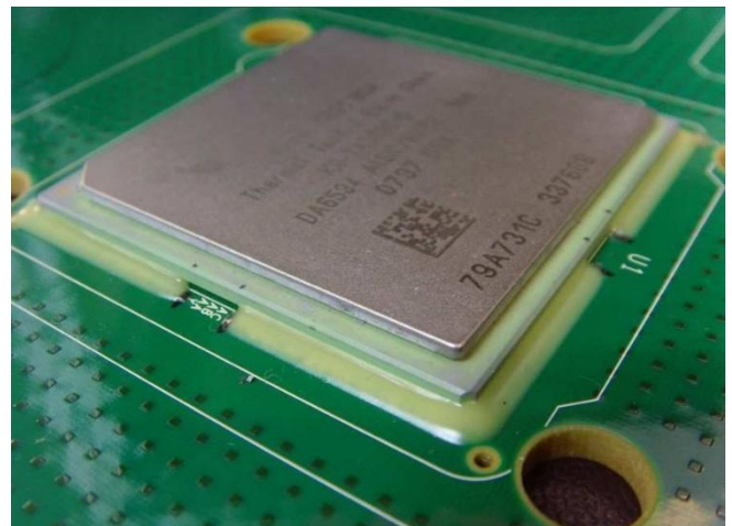
Figure 1. Edgebonded CBGA, courtesy of Celestica, Inc.
